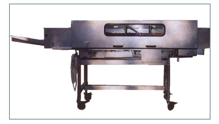
The Gutting Units SGA-22 & SGA-32 are salmon gutting units. The system includes an active cutting system to enable removal of roe and/or viscera without the need for pre-bulleting.
